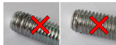
Fig 3 damaged M10 screws
