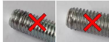
Picture 5 damaged M10-bolts
